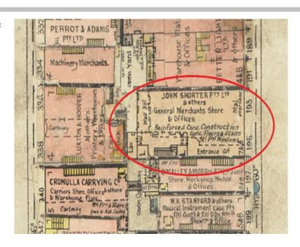
Caption: Undated Fire Underwriter's plan recording details of the building height, construction and
