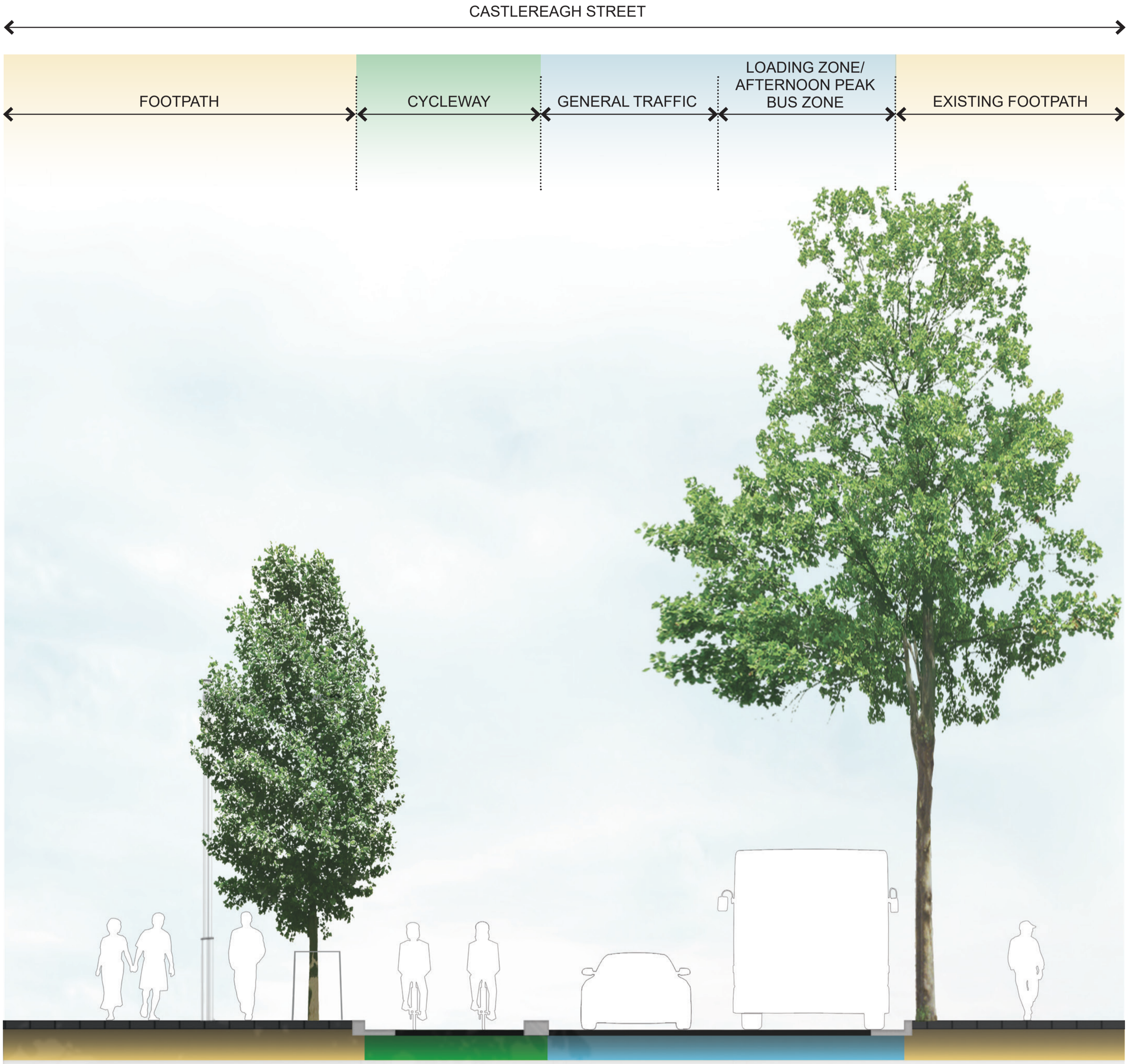
TYPICAL STREET CROSS SECTION A-A CASTLEREAGH STREET BETWEEN LIVERPOOL STREET AND BATHURST STREET
