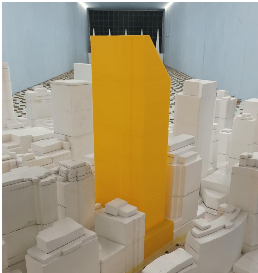
Figure 2a: Photograph of the Wind Tunnel Model Envelope Case, view from the north-west
