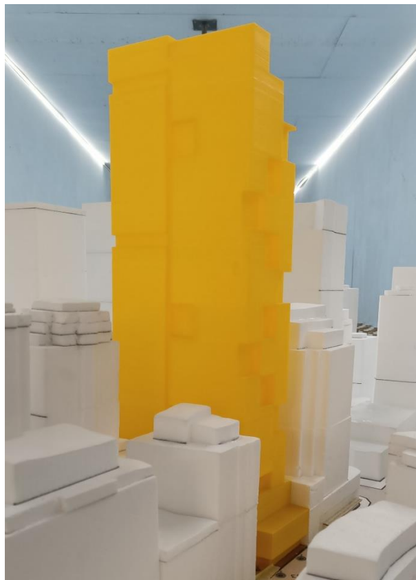
Figure 2a: Photograph of the Wind Tunnel Model Massing Case, view from the north-west
