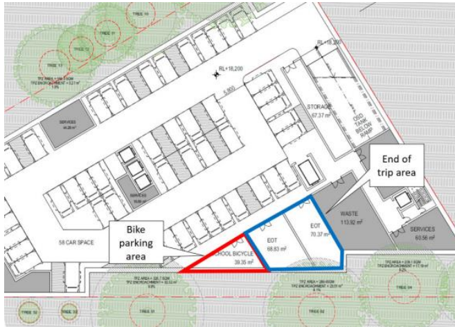
Figure 41 Bicycle parking and end of trip facilities
