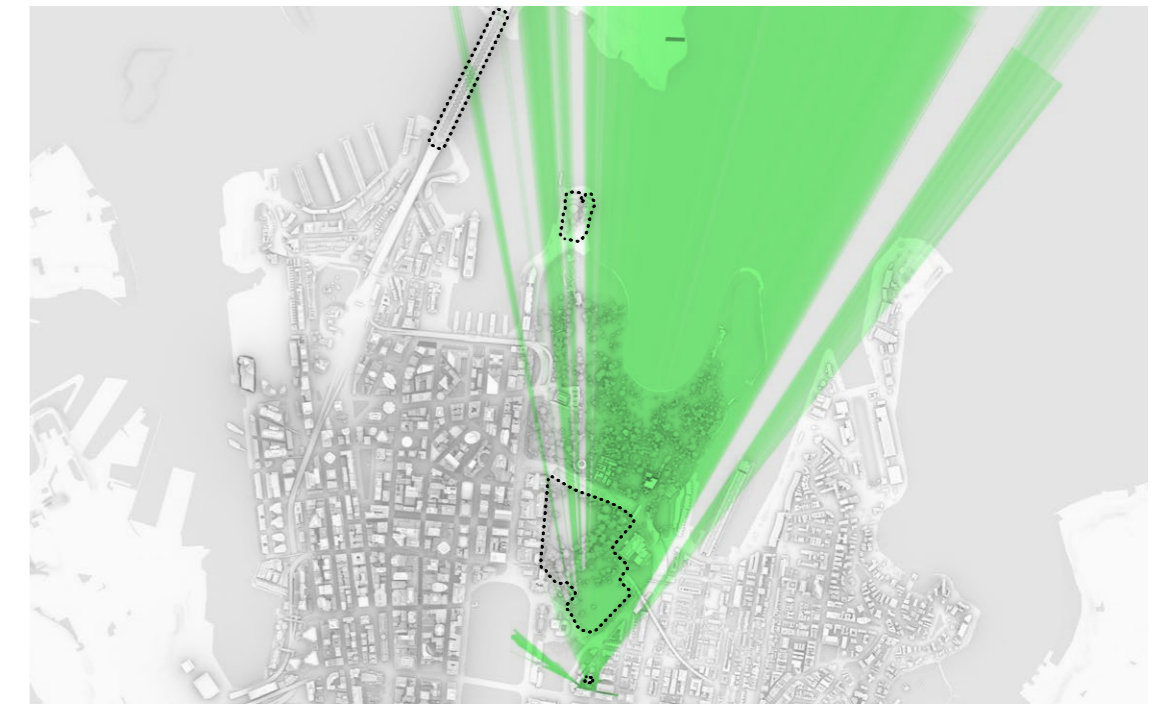
The diagram above depicts the view of an apartment on the 7th floor of 60-70 William St with the proposed envelope introduced. The field of view of a person is simulated, showing how views are impacted by the proposed envelopes, existing buildings and trees.
