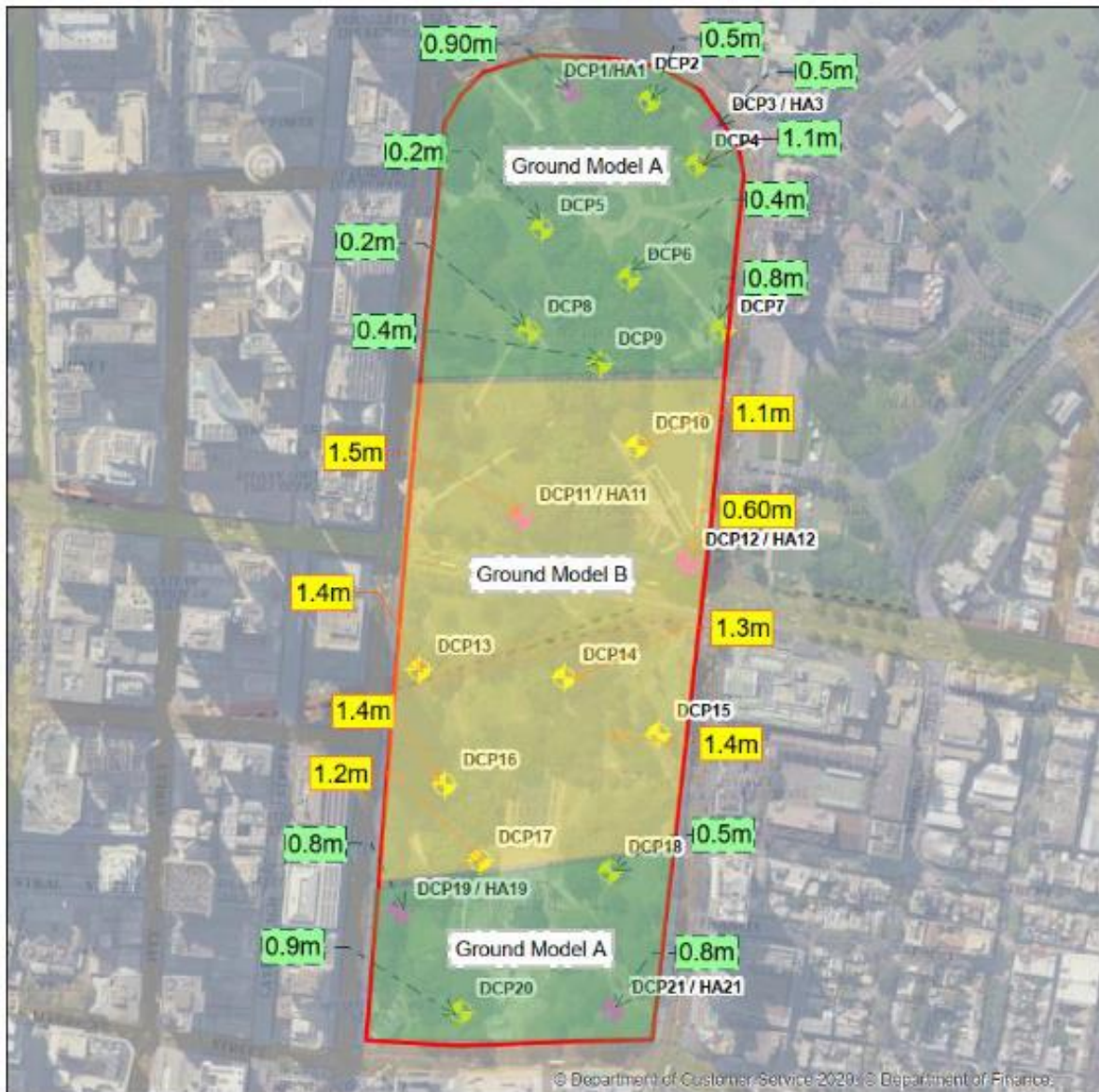
Figure 4.5 Plan showing geotechnical Ground Model Areas A and B with DCP and hand auger locations. (Source: AECOM 2021:6)
