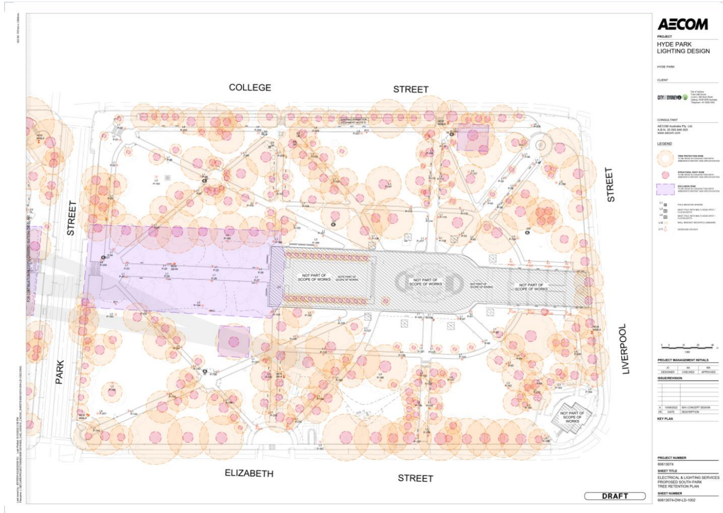
Figure 6-13 TPZ/SRZ of trees present within Hyde Park South
