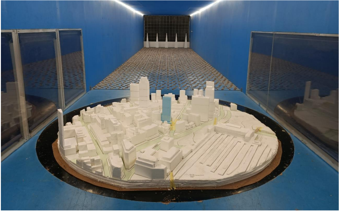
Figure 1e: Photograph of the Wind Tunnel Model (Proposed Case, view from the south)
